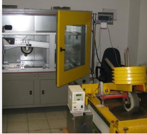
Hamburg Device: Steel Wheels in Water Bath at 50°C
